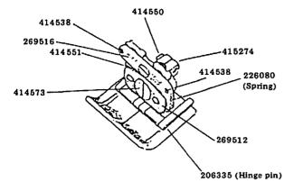
PART NO.DESCRIPTION206335Presser Foot Hinge Pin226080Presser Foot Plate Spring269512Presser Foot Shank Guide Plate414538Presser Foot Bracket Guide Screw (2)414550Presser Foot Bracket Pintch Screw414551Presser Foot Shank Guide Plate Hinge Screw414573Presser Foot Shank Guide Plate Hinge Screw41573Presser Foot Shank Guide Plate Hinge Screw415274Presser Foot Bracket with 414550
